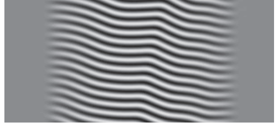
Fig. 3: Stripes favour a perpendicular orientation with respect to shallow control parameter drops ( \delta_x = 5\lambda_c ). Simulation of the Brusselator started at \beta_m = 0.001 and was slowly increased to \beta_m = 0.05 . Parameters: l_x = l_y = 50\lambda_c , N_x = N_y = 1024 . Note: only a cutout of the simulation is shown.
