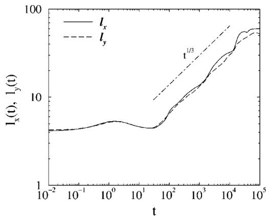
FIG. 3. Dynamics of the characteristic length scales  $l_x(t)$  and  $l_y(t)$  without driving ( $a=0$ ). System size  $L_x=L_y=256$ ,  $\epsilon=1$ .
