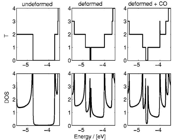
FIG. 10. DOS and transmission per spin for the semiconducting (8, 0) CNT. Left: undeformed, middle: deformed, and right: deformed with attached CO molecule.
