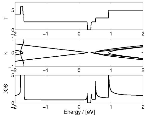
FIG. 7. Band structure, DOS, and transmission per spin for a zigzag (6, 0) tube using  $sp^3$  orbitals. The “metallic” tube becomes semiconducting with a band gap of  $\approx 0.1$  eV and shift of the Fermi level from 0.0 to  $\approx 0.3$  eV.
