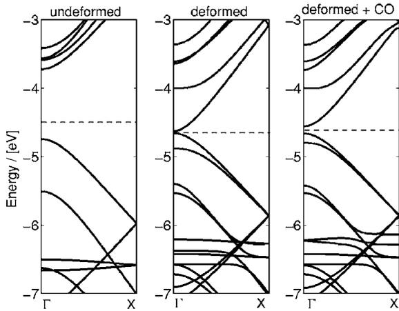
FIG. 9. Band structures of a zigzag (8, 0) CNT using  $sp^3d^5$  orbitals. Left: undeformed tube with a band gap of  $E_G \approx 1.1$  eV, middle: deformed tube with a small gap of  $E_G \approx 25$  meV, and right: deformed tube with attached CO molecule at distance 1.85 Å. The gap here is  $E_G \approx 100$  meV. The Fermi energy is indicated by the dashed line.
