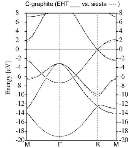
FIG. 2. 2D band structure of a graphene sheet along the  $M \rightarrow \Gamma \rightarrow K \rightarrow M$  path within the first Brillouin zone. The solid line corresponds to the EHT band structure using parameters optimized to match the DFT-GGA band structure (dashed line), see Refs. 22 and 23. The C-C bonding distance is set to  $a_{C-C}=1.44 \text{ \AA}$ , and the cutoff radius for the neighbor atoms is  $R_c=9 \text{ \AA}$ . The Fermi level is at  $E_F=0.0 \text{ eV}$ .
