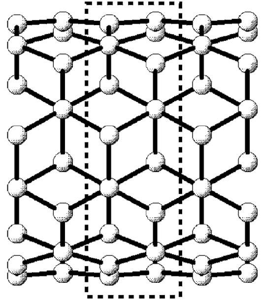
FIG. 1. Sketch of a (5, 5) armchair tube with three unit cells. The dashed rectangle marks the center unit cell containing 20 carbon atoms. For the calculation of the  $E$ - $k$  dispersion we use the first nearest-neighbor unit cells to the left and right, respectively.
