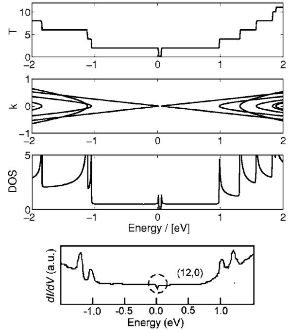
FIG. 4. Band structure, DOS, and transmission per spin for a “metallic” zigzag (12, 0) tube using  $sp^3$  orbitals. The gap close to the Fermi level at  $E_F=0.0$  eV is about 50 meV. For comparison the experimental STS- $dI/dV$  signal is shown at the bottom (Ref. 34). The bottom figure has been reprinted with permission from Ref. 34. Copyright 2001 American Association for the Advancement of Science.
