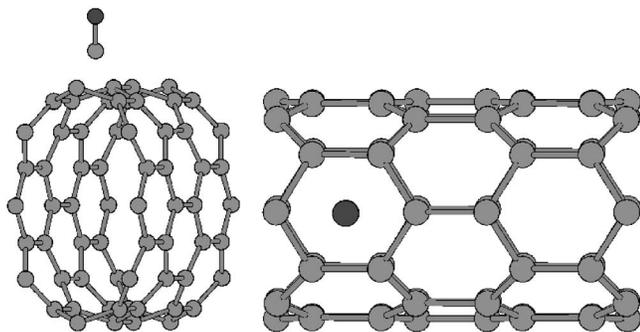
FIG. 8. Unit cell of a semiconducting (8,0) CNT with one CO molecule at distance of  $d=1.85$  Å from the CNT surface. The CO molecule has been placed above the center of the hexagon which is the most stable equilibrium position after relaxation (Ref. 24). The unit cell of the periodic structure consist of two (8,0) CNT unit cells and one CO molecule, i.e., the cell contains 66 atoms.
