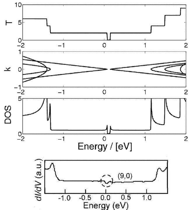
FIG. 5. Band structure, DOS, and transmission per spin for a “metallic” zigzag (9, 0) tube using  $sp^3$  orbitals. The gap close to the Fermi level at  $E_F=0.0$  eV is about 80 meV similar to STS- $dI/dV$  measurements as shown at the bottom (Ref. 34). The bottom figure has been reprinted with permission from Ref. 34. Copyright 2001 American Association for the Advancement of Science.
