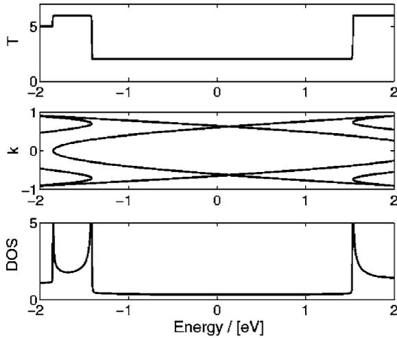
FIG. 3. Band structure, transmission, and DOS per spin for an armchair (5, 5) tube using  $sp^3$  orbitals. Due to their mirror symmetry the curvature of the tube does not break this symmetry, so that the tube remains strictly metallic. The Fermi level is  $E_F=0.0$  eV and  $k$  is in units of  $\pi/T_0$ .
