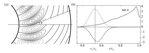
FIGURE 6. For  $E=2\times 10^{-5}$ ,  $\epsilon=0.01$ , with the QG model, i.e. for the wave already displayed in figure 5(e). (a) Zoom on the contours of  $v_r$  showing the tilt angle at the critical radius  $r_c$ . (b) The dotted line shows the factor  $E_{cr}/2$ , the thin line the slope  $\tan \alpha$ , the dashed line illustrates (3.20) by showing the product  $-E_{cr} \tan \alpha$ , i.e. half the Reynolds stress  $\tau_{r\varphi}$ .
