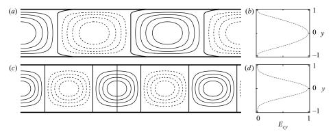
FIGURE 2. (a) Streamlines of the critical Tollmien–Schlichting wave flow v (see (2.1)). (b) Corresponding transverse kinetic energy  $E_{cy}$ . (c,d) Same plots for the Rayleigh–Bénard convection rolls. The grey line in (c) shows the mirror advocated in (2.11).
