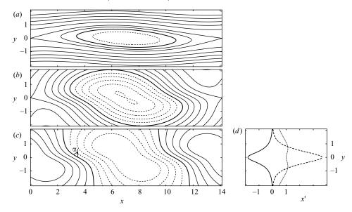
FIGURE 4. Most-amplified Kelvin–Helmholtz wave destabilizing the shear-layer profile (2.18). (a) Streamlines of the total flow  $V_0 + v$ , with a wave-amplitude A = 0.1. (b) The same, but with a larger wave amplitude A = 1. (c) Streamlines of the wave flow  $v_1$  alone, i.e. ' $A = \infty$ '. (d) Kinetic energy  $E_{cy}$  (dotted line), slope  $x_s'$  (continuous line) and Reynolds stress  $\tau_{xy}$  (dashed line).
