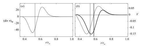
FIGURE 7. For the conditions of figure 6, with the two-dimensional (thin lines) or three-dimensional (thick line) models. (a) Azimuthal component of the divergence of the Reynolds-stress tensor, the right-hand side of (3.21). (b) Zonal flow profiles in the equatorial annulus. The vertical lines show  $r_c^{2D}/r_o$  and  $r_c^{3D}/r_o$ .
