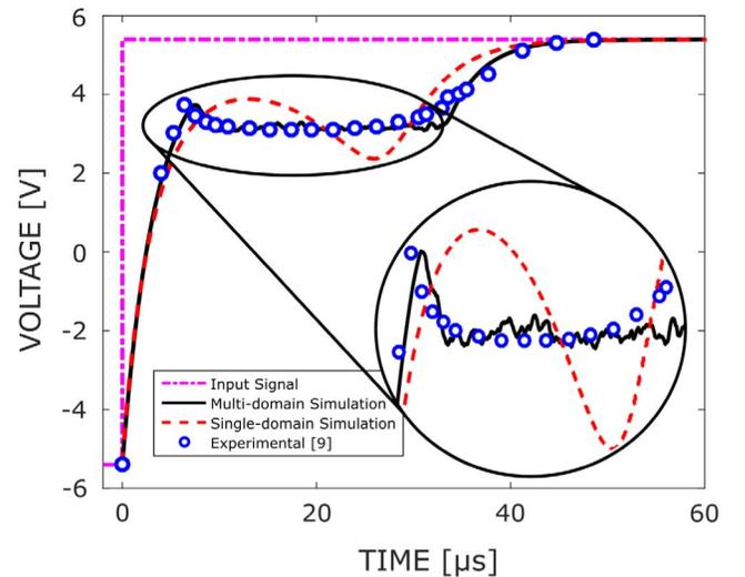
Fig. 4. Validation of our simulation methodology via a comparison with the experimental curves in [16]. Circles show experimentally measured values for the voltage  $v_{FE}$  across the ferroelectric. Solid line shows the result of our multidomain simulation, which exhibits a strong match to experiment. Dashed lines show the result of a single-domain simulation. The input voltage is also shown as a dashed-dotted line.
