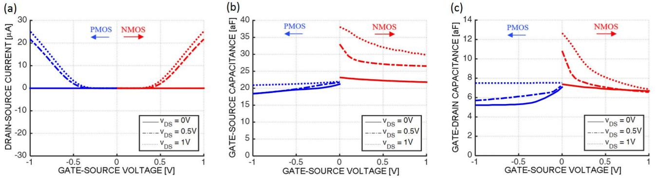
Fig. 3. Cadence Spectre [22] simulation results for a 28-nm FET. (a)  $i_{DS}(v_{GS}, v_{DS})$  curves of nMOS and pMOS. (b)  $C_{GS}(v_{GS}, v_{DS})$  curves for nMOS and pMOS. (c)  $C_{GD}(v_{GS}, v_{DS})$  curves for nMOS (red online) and pMOS (blue online).
